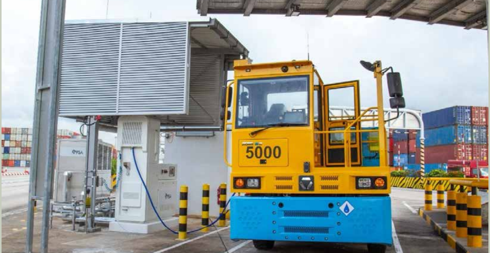
Hydrogen fuel cell electric prime mover refuelling at Pasir Panjang Terminal
